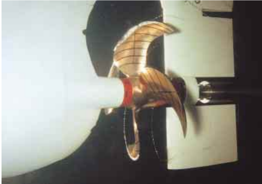
Model test of a high skew propeller for a single screw 16000 DWT tanker.
