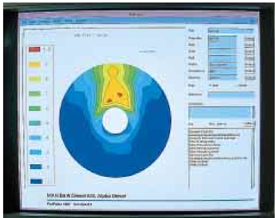
Full scale wake field calculated from model wake field.
