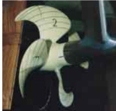
Model test of a high skew propeller for a twin screw 3990 GT cruise vessel.
