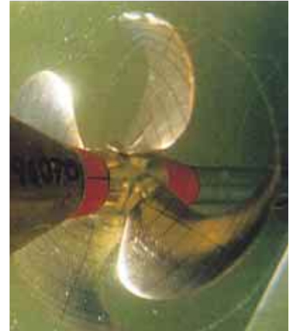
Model test of a high skew propeller for a single screw 5100 DWT chemical tanker.
