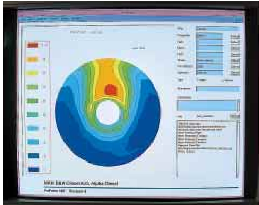
Measured wake field in model scale.
