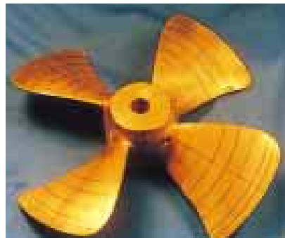
The AHTS model propeller.
