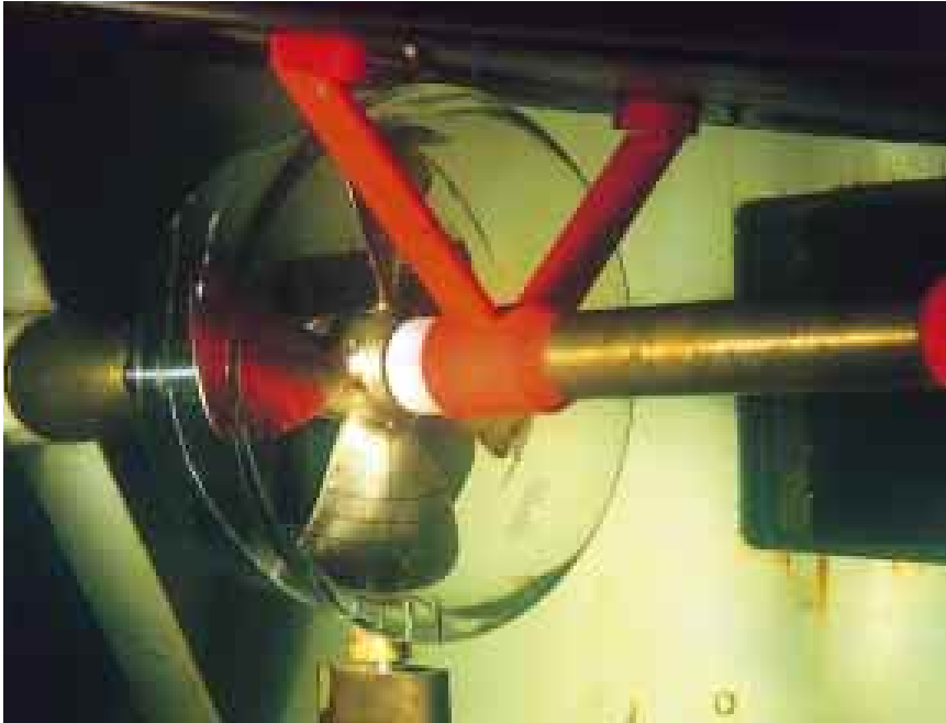
Model test of a ducted propeller for a twin screw AHTS vessel.
